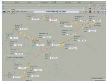
Citect SCADA Gas Control Page and Overview of Northern Region Gas Network
